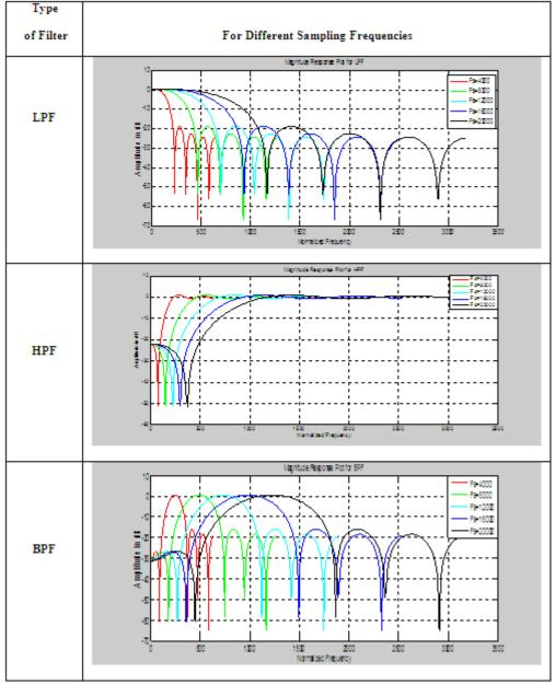
Figure: Magnitude Response Curves for FIR Filters for different sampling frequencies
